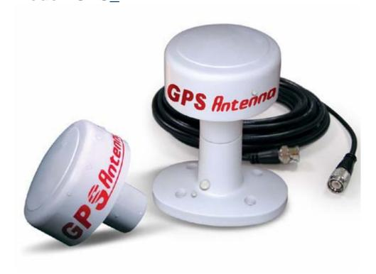
Supply Voltage 5.0 V DC Current Consumption 18mA@ 5.0V DC VSWR 1.5 max. Output Impedance 50 ohm Center Frequency 1575.42 MHz Gain 30 +/-4.5dB Noise Figure 2.0 max Bandwidth 2 MHz min.
